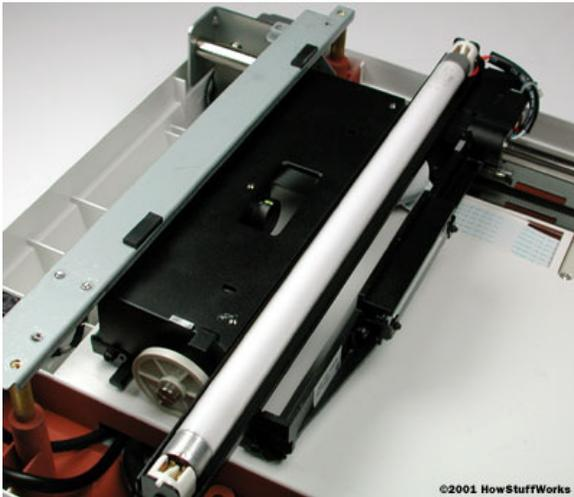
In the image above, you can see the fluorescent lamp on top of the scan head.
