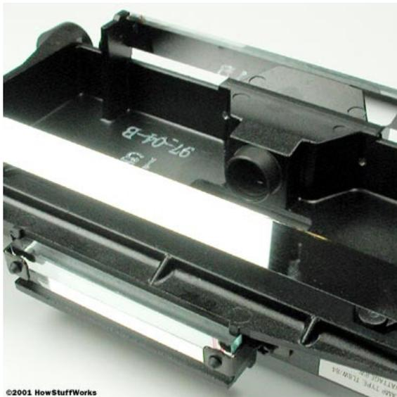
Look carefully at the image above and you can see all three of the mirrors plus the lens assembly in this scan head.
