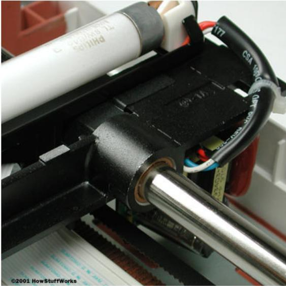
The stabilizer bar is very durable and tightly secured to the body of the scanner.
